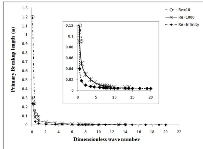
Fig. 3. The Effect of Liquid Viscosity on the primary break up of spray at  $We_l=We_s=1000$ ,  $g_i=g_o=0.00123$ ,  $h=0.95$
