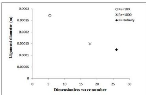
**Fig. 11.** The Effect of Liquid Viscosity on Ligament diameter at  $We_i=We_s=1000$ ,  $We_i=We_o=We_{si}=We_{so}=30$ ,  $g_i=g_o=0.00123$ ,  $h=0.95$
