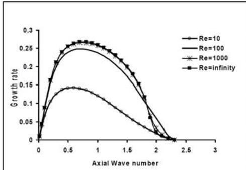
Fig. 2. Dispersion diagram at  $We_l=1000$ ,  $g_i=g_o=0.00123$ ,  $h=0.95$
