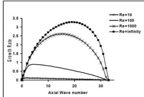
Fig. 3. Dispersion diagram at  $We_l=We_s=1000$ ,  $g_i=g_o=0.00123$ ,  $h=0.95$
