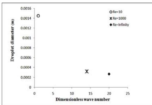
Fig. 4. The Effect of Liquid Viscosity on Droplet diameter at  $We_l=We_s=1000$ ,  $g_i=g_o=0.00123$ ,  $h=0.95$
