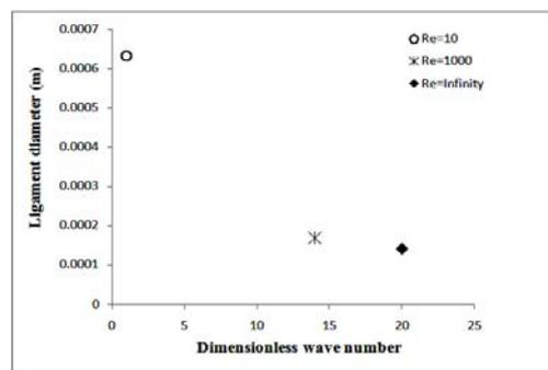
Fig. 5. The Effect of Liquid Viscosity on Ligament diameter at  $We_l=We_s=1000$ ,  $g_i=g_o=0.00123$ ,  $h=0.95$
