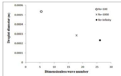
**Fig. 12.** The Effect of Liquid Viscosity on Droplet diameter at  $We_i=We_s=1000$ ,  $We_i=We_o=We_{si}=We_{so}=30$ ,  $g_i=g_o=0.00123$ ,  $h=0.95$
