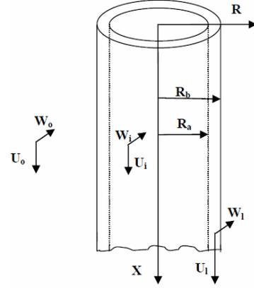
**Fig. 1.** Annular swirling viscous liquid sheet subject to swirling airstreams
