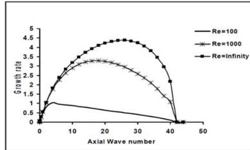
**Fig. 9.** Dispersion diagram at  $We_i=We_s=1000$ ,  $We_i=We_o=We_{si}=We_{so}=30$ ,  $g_i=g_o=0.00123$ ,  $h=0.95$
